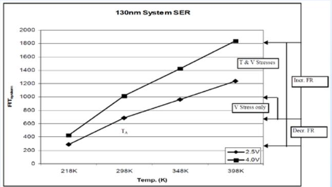
*Part degradation Acceleration Factors and Derating Factors may be calculated as a function of Temperature and Voltage for a given application.*
