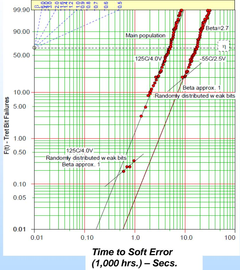
**The main population at 90nm is tighter than at 130nm. Also the margin in weakest bits is improved at 90. This sort of trend is expected to continue to smaller feature sizes.**
