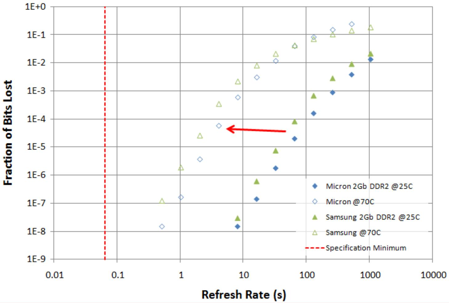
***Elevated temperature results in much faster data loss – this effect drives datasheet refresh requirement.***
